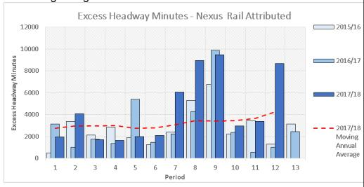
Excess Headway Minutes (Network Rail) An average of just under 1,000 EHM per four-week period were allocated to Network Rail, this is an improvement of over 200 EHM per four-week period when compared with the previous three periods and an improvement of over 700 EHM per four-week period when compared with the same time last year. A signalling fault on 10 December 2017 accounted for the higher than normal EHM levels during Period 10.
